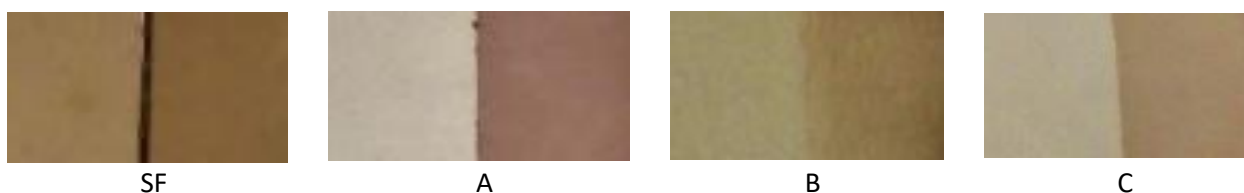
Figure 2. Leather SF, A, B and C before and after ageing after the dry heat ageing at 120° C for 96 hours.
